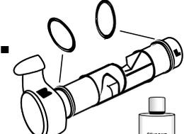
Replace both O-rings. Apply silicone lubricant that came with your FROG Leap Infuzer on O-rings.
