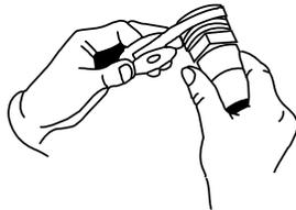
2. Screw adapters into each end of FROG Leap Infuzer. Hand tighten. Finish tightening by turning 1 to 2 revolutions with pipe wrench. **DO NOT OVER TIGHTEN.**
