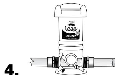
4. Insert PVC pipe into adapters with a twisting action. Hold in place 5 to 10 seconds to bond.
