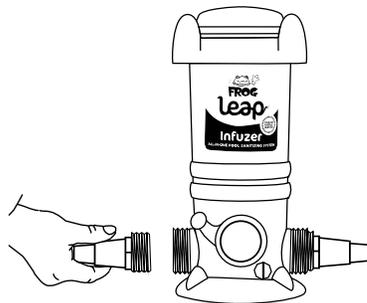
3. Attach the filter section of flex hose to one hose adapter and the return section of flex hose to the other hose adapter with clamps and tighten with screwdriver. Bi-flow valve design allows water flow installation in either direction.
