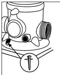
For better stability, FROG Leap Infuzer may be mounted on a treated wood base using **Phillips pan head screws**, one in front and two in back. If you have questions about stability, please contact your dealer or King Technology.
