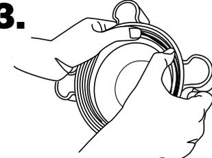
Place your thumbs on each side of the cap over the O-ring in the groove.
