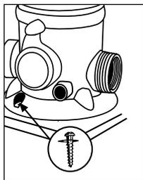
For better stability, FROG Leap Infuzer may be mounted on a treated wood base using **Phillips pan head screws**, one in front and two in back. If you have questions about stability, please contact your dealer or King Technology.
