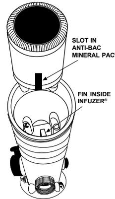
Find slot on side of FROG Leap Anti-Bac Mineral Pac and line up with fin inside the FROG Leap Infuzer. Lower FROG Leap Anti-Bac Mineral Pac into FROG Leap Infuzer until secure.
