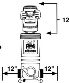
Allow a minimum of 12" above and on each side of FROG Leap Infuzer to ensure room for easy replacement of FROG Leap Anti-Bac Mineral Pac and FROG Leap Torpedo Pac.
