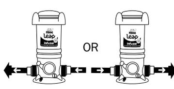
Bi-flow valve design allows installation in either flow direction.
