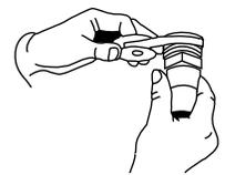
**5.** Screw adapter into the other side of FROG Leap Infuzer. Hand tighten. Finish tightening by turning 1 to 2 revolutions with a pipe wrench. **DO NOT OVER TIGHTEN.**
