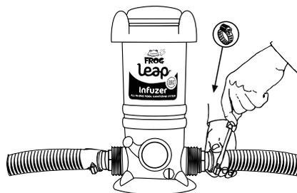
4. To prevent damage to heaters or filters, install a **corrosion resistant check valve** which will reduce the back flow of chlorine gas when the system is turned off.
