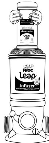
Line up the small leg of the FROG Leap Depth Charge or Reveille with the small opening in the FROG Leap Anti-Bac Mineral Pac and the large leg with the large opening. Lower pac into FROG Leap Anti-Bac Mineral Pac until secure.
