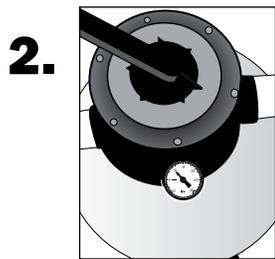
**2.** Check the pool's filter gauge often and periodically clean filter per the manufacturer's directions. A dirty filter will slow the flow of water which could hamper proper circulation.
