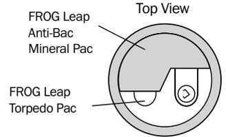
**5.** Replace cap by hand only. **DO NOT OVER TIGHTEN.**
