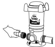
**6.** Attach return section of hose to the adapter with clamp. Tighten clamp with screwdriver.
