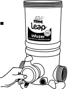
Carefully insert control dial back into housing.
