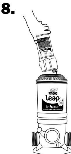
Lift FROG Leap All-Out up and allow any water in the container to drain through the FROG Leap Infuzer before discarding in trash or offering for recycling. Do not reuse or refill this container.
