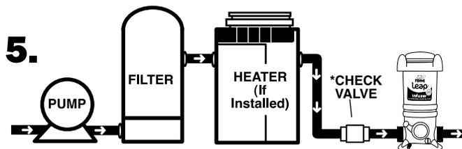
5. To prevent damage to heaters or filters, see your dealer about installing a **corrosion resistant check valve** which will reduce the back flow of chlorine gas when the Infuzer is turned off.
