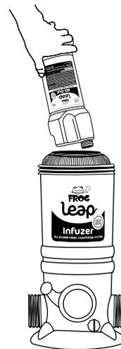
Insert FROG Leap All-Out into the open center of the FROG Leap Anti-Bac Mineral Pac in the Infuzer. (See page 17 for directions.)
