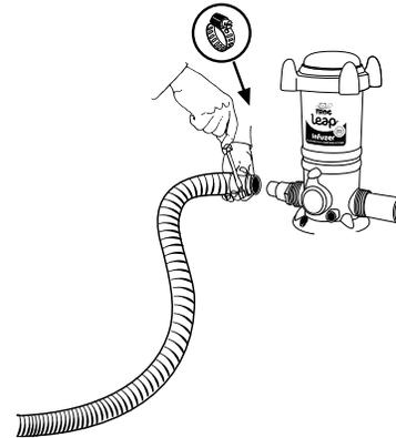
**7.** To prevent damage to heaters or filters, see your dealer about installing a **corrosion resistant check valve** which will reduce the back flow of chlorine gas when the FROG Leap Infuzer is turned off.
