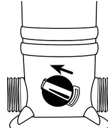
Replace locking pin by pushing it through the slots on the dial until it locks into place.
