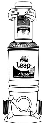
When chlorine reading is down to 1.0 ppm, which may take a few days, insert FROG Leap Torpedo Pac into the open center of the FROG Leap Anti-Bac Mineral Pac. (See page 18 for directions.)
