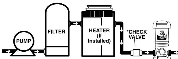
The FROG Leap Infuzer should always be installed between the filter and pool (or between heater and pool if applicable). Never install FROG Leap Infuzer before the heater or damage to the heater could occur.
