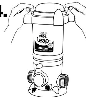
Replace cap by hand only. **DO NOT OVER TIGHTEN.**
