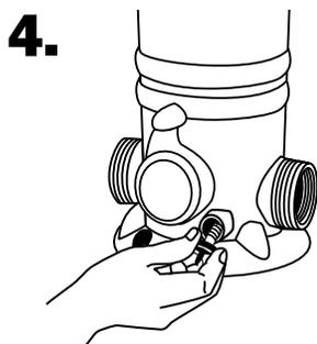
Unscrew knob from the front of FROG Leap Infuzer. Allow all water to drain.
