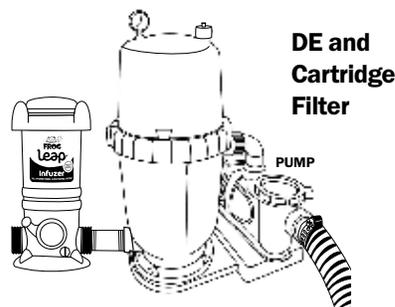
**4.** Apply pipe thread tape or sealant to threaded end of hose adapter.
