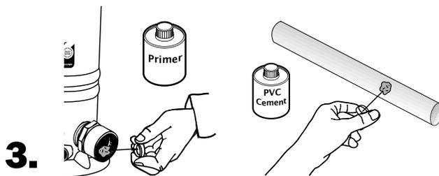
3. Following Primer directions, brush Primer on the inside of the adapters and to ends of pipe. Repeat this process with PVC cement following manufacturer's directions on that product.
